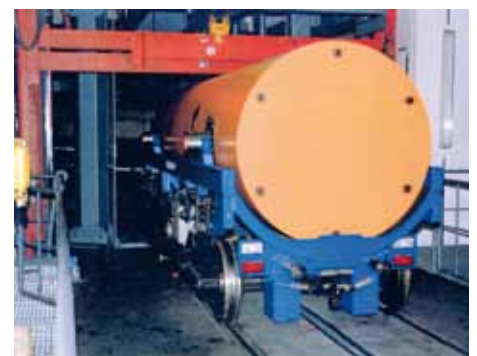
Demonstration test for the shaft hoisting of a POLLUX® cask
