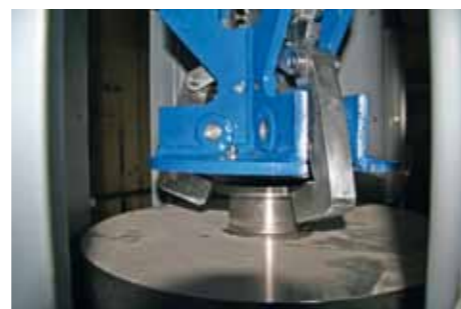
Demonstration test for retrieval of a spent fuel canister (bottom) from a borehole by a grabber. Landesbergen (Germany)
