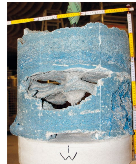
Sample of crushed salt grouted with MgO-water glass mixture (marked in blue)
