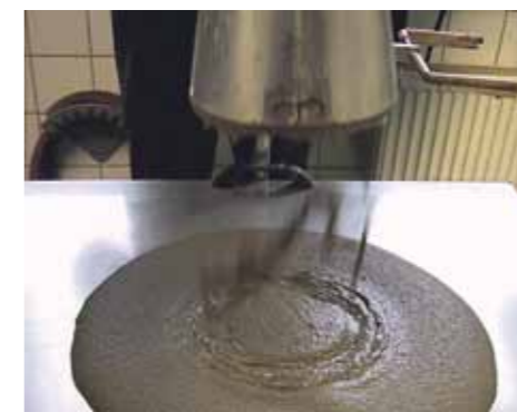
Slump test for concrete analysis
