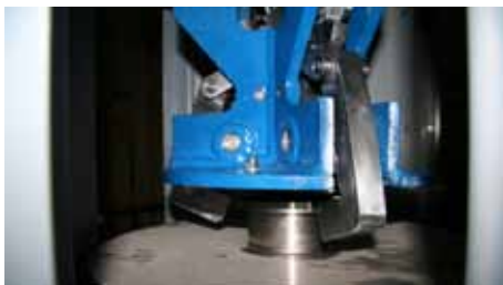
Demonstration test for borehole emplacement: The spent fuel canister (below) can be caught by a grabber and retrieved from the borehole.
